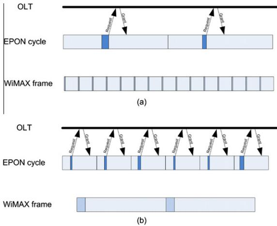
Fig. 3. EPON cycle in comparison with WiMAX frames.
