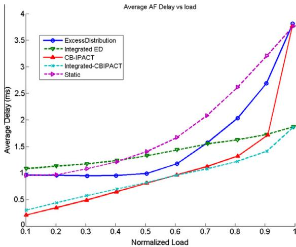
Fig. 10. Delay of AF flow in different loads.
