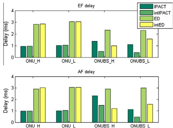
Fig. 22. The delay of EF and AF traffic classes in realistic scenario [added].
