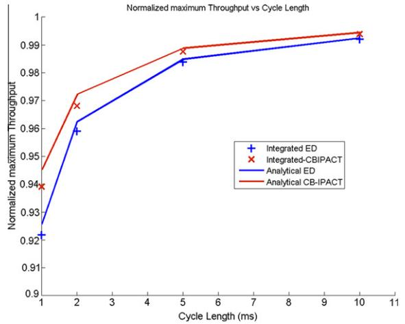
Fig. 14. Normalized analytic throughput versus cycle length.
