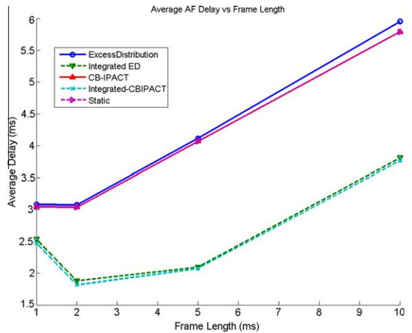
Fig. 21. AF stream delay versus frame length.
