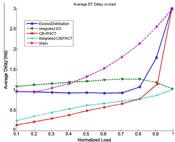
Fig. 9. Delay of EF flow in different loads.
