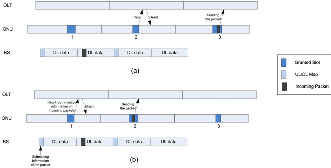
Fig. 2. Timing diagram of sending a marked packet (a) normal scheduling (b) integrated scheduling [moved accordingly].
