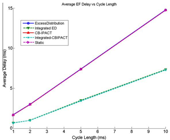
Fig. 15. EF stream delay versus EPON cycle length.
