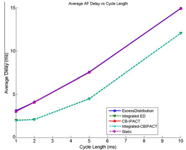
Fig. 18. AF stream delay versus EPON cycle length.
