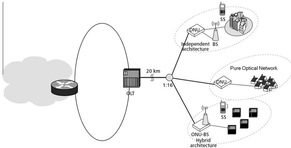
Fig. 1. Integrated EPON and WiMAX architectures [27] [moved accordingly].
