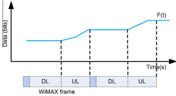
Fig. 4. Relationship between  $F(t)$  and WiMAX frame.
