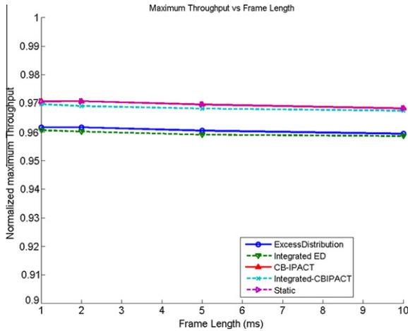
Fig. 19. Maximum throughput versus frame length.
